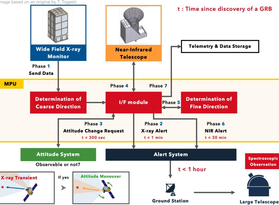
Our objective is to disseminate information regarding high-redshift GRBs to the community all over the world quickly as possible. To achieve this, it is important to analyze WFXM and NIRT data on the satellite. The Mission Processing Unit (MPU), on-board system of the satellite, receives science data from these mission instrument and analyzes them. Also, the MPU would launch some commands to mission instrument. The figure on the left shows the rough observation process of HiZ-GUNDAM.
