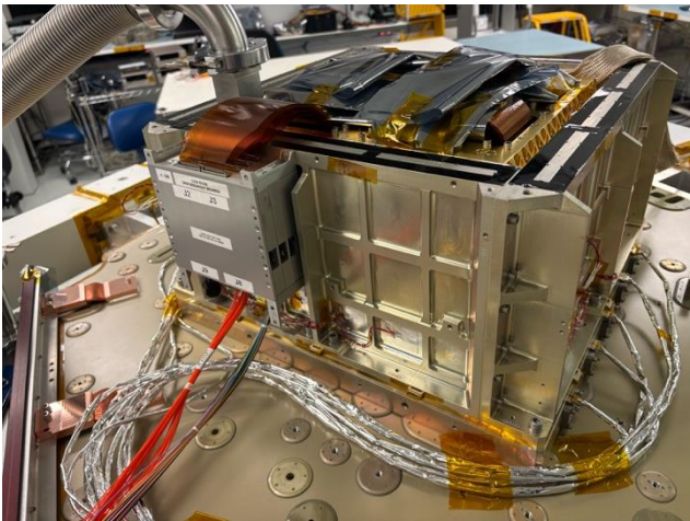
Doing electrical checks after adding cryostat shell and ACS
