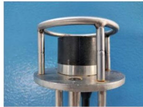
Transmitters are deployed at string junction boxes
