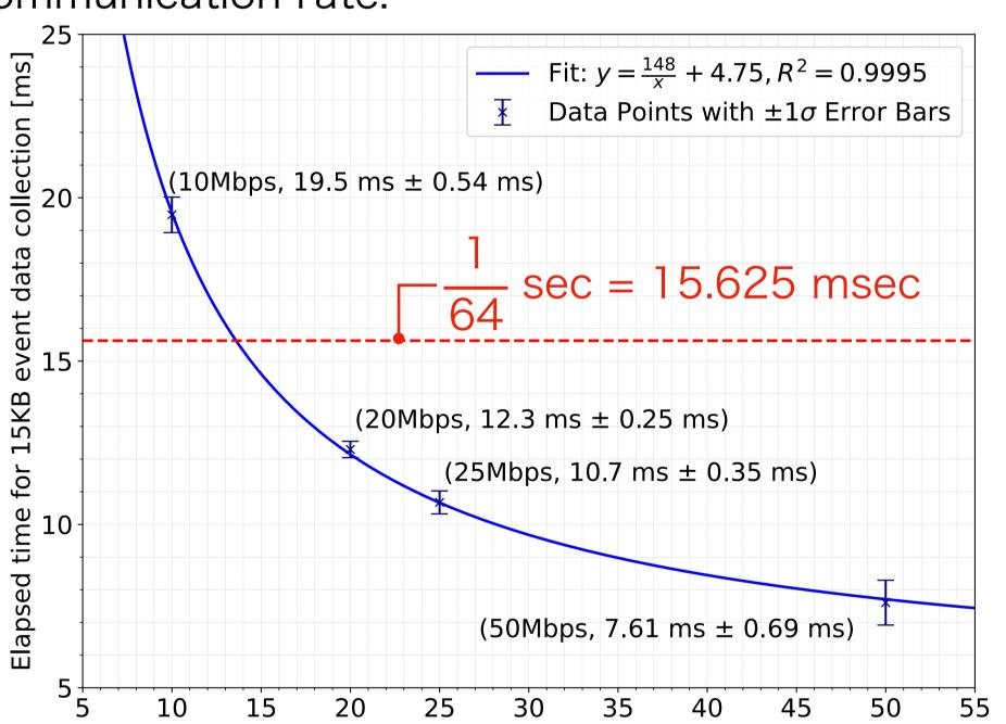
The graph on the left shows the elapsed time for data collection by one module. It shows that the required time decreases in inverse proportion to the set communication rate.
