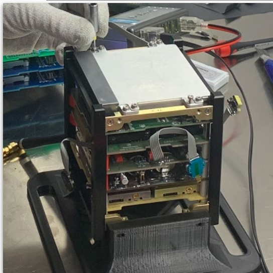
GRB Alpha (2021.03-2024.06); 1U-sized prototype satellite ( https://grbalpha.konkoly.hu/ ) • has smaller detector, but the same basic concept T. Mizuno
