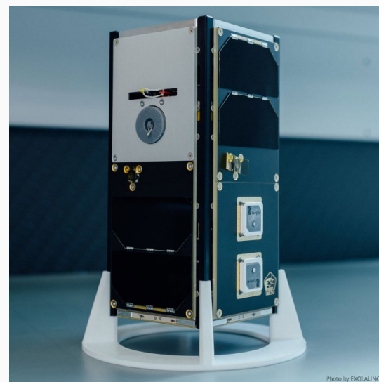
GRB beta (2024.07-); 2U-sized technological precursor ( https://grbbeta.tuke.sk/index.php/en/ ) • tests several technologies such as attitude control and UV camera
